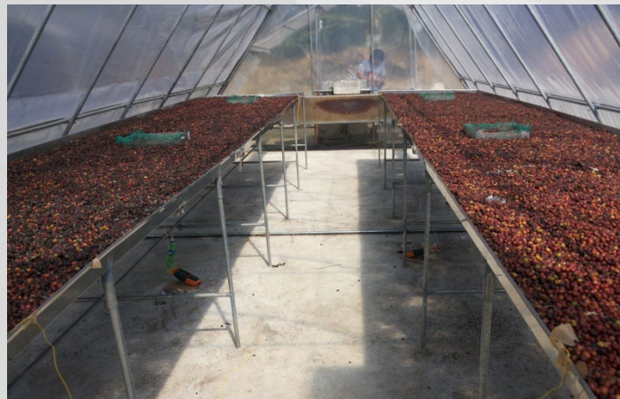
Field testing of improved Greenhouse-Type Solar Dryer for coffee
