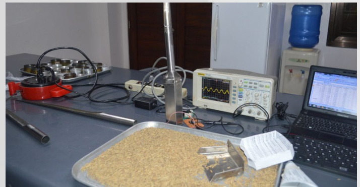
Actual laboratory testing of probe moisture content meter
