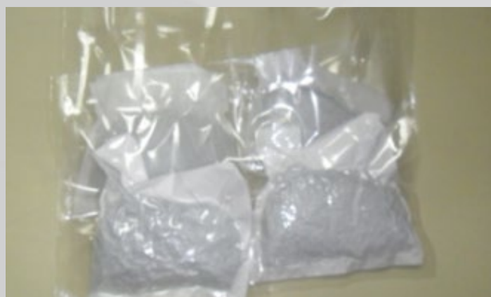
Silica gel packed in permeable paper (6.5 x 15.5cm) and sealed with second layer of non-permeable plastic film (oriented polypropylene/cast).
